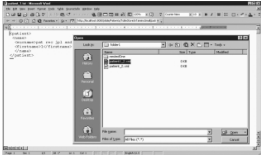
Editing of Web-documents in Word 2000 – here an XML document stored in Software AG's native XML Database Tamino on a remote Web-server – is the same as editing local documents. Just open a Web folder, double click the document, edit, and press the Save button.
